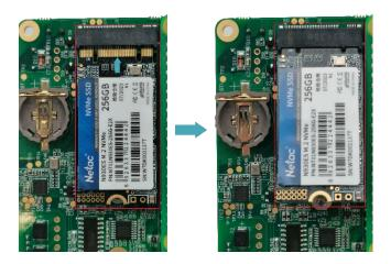
3. Insert the screws that secure the SSD and tighten clockwise to secure the SSD to the PCBA.
