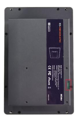
2. Insert the SD card into the corresponding card slot with the contact side facing down, making sure it will not fall out.
