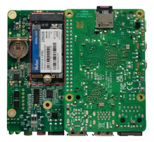
2. Use a screwdriver to loosen the screws that secure the SSD counterclockwise.
