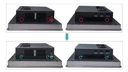
4. Align the ports on the PCBA with the port's holes on the side panel, and insert the side cover.
