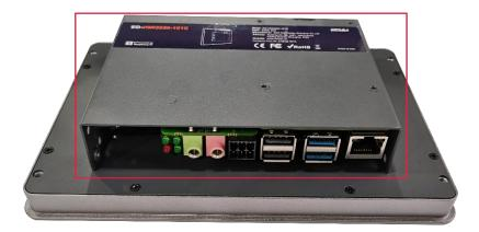
3. Use a screwdriver to tighten four M3 screws and one grounding screw on two sides clockwise.
