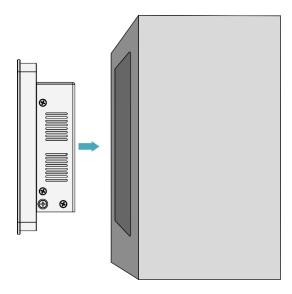
4. Align the screw hole (unthreaded hole) of the buckle with the buckle mounting hole on the side of the device.
