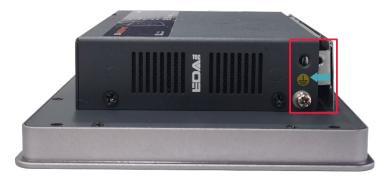
5. Use a screwdriver to tighten 2 M3 screws clockwise to fix the side cover.
