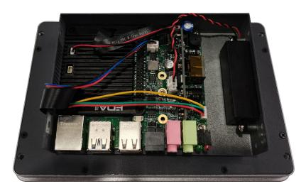
6. Use a screwdriver to loosen 6 screws of PCBA mounting counterclockwise to separate the PCBA from the metal case, and flip it to the back of PCBA.
