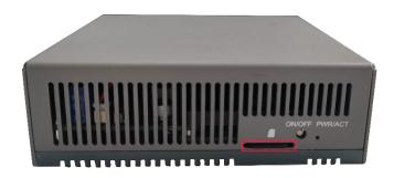
2. Use tweezers to hold the SD card and pull it out.
