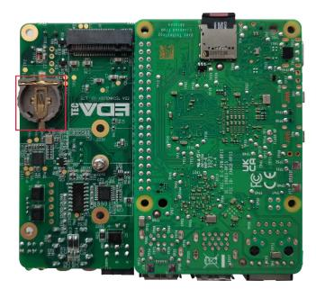
2. Place the positive terminal of the battery facing up, and press it into the RTC base. The completed installation is as shown below.
