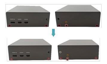
4. Align the interface on the PCBA with the interface holes on the front panel, insert the front cover, and then use a screwdriver to tighten the 2 M3 screws clockwise.
