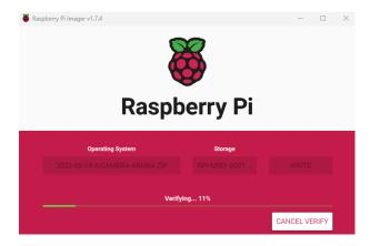
7. After the file verification is completed, the prompt box "Write Successful" pops up, and click "CONTINUE" to finish flashing SD card.
