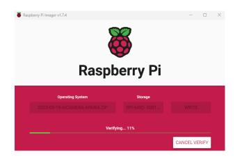
7. After the file verification is completed, the prompt box "Write Successful" pops up, and click "CONTINUE" to finish flashing SD card.
