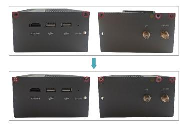
3. Align the ports on PCBA with the ports on the front panel, insert the front cover, and then use a screwdriver to fasten two M3 screws clockwise, as shown in the following figure.
