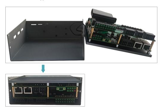
2. Align the screw holes on the upper and side panels, and use a screwdriver to tighten four M2.5 screws and one grounding screw on two sides clockwise, as shown in the following figure.
