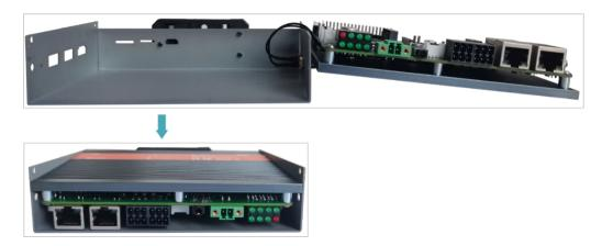
Align the screw holes on the upper and side panels, and use a screwdriver to tighten four M2.5 screws and one grounding screw on two sides clockwise, as shown in the following figure.
