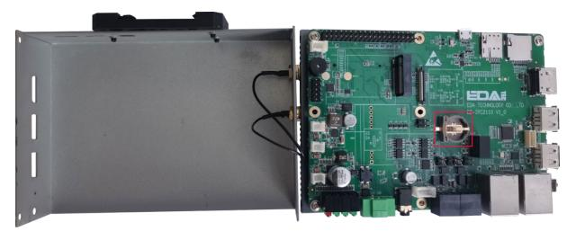
Put the positive pole of the battery upwards and press it into the RTC base. The installation effect is as shown below.
