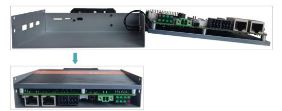
Align the screw holes on the upper and side panels, and use a screwdriver to tighten four M2.5 screws and one grounding screw on two sides clockwise, as shown in the following figure.
