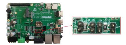
The corresponding relationship between  $120\Omega$  terminal resistance and serial port is as follows:
