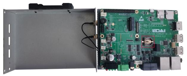
2. Put the positive pole of the battery upwards and press it into the RTC base. The installation effect is as shown below.
