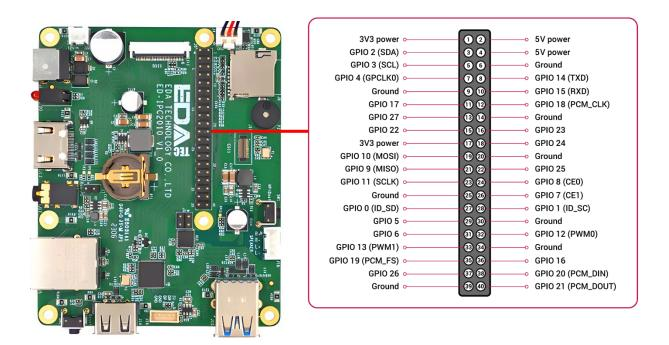
There is a debugging serial port in ED-IPC2000 series 40Pin, and GPIO14 GPIO15 are read and write pins respectively.
